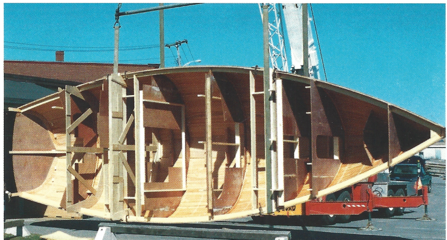
Turning of the hull: GUSTO, Paine 44, cold molded cruiser under construction at French & Webb will be fitted with GMT spars.
