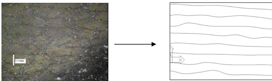
Figure 4b: microstructure of a M46J autoclave sample
