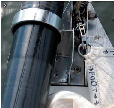
❸ The pole's forward end slides through a Delrin sleeve inside a stainless ring secured to the stemhead fitting. ❹ Both owners also wanted to be able to continue to use their symmetric chutes and mast-ended poles. ❺ When the pole is deployed, the after end secures with a simple quick-release pin, a manual and nearly foolproof system.
